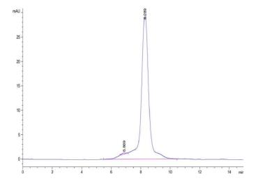
The purity of Canine IL-23R is greater than 95% as determined by SEC-HPLC.
